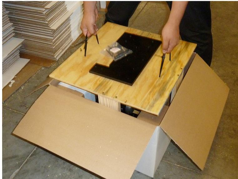
Fig. 1—Lifting out the shipping frame using the zip tie handles.
