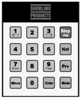
Figure 2—Layout of the keypad
