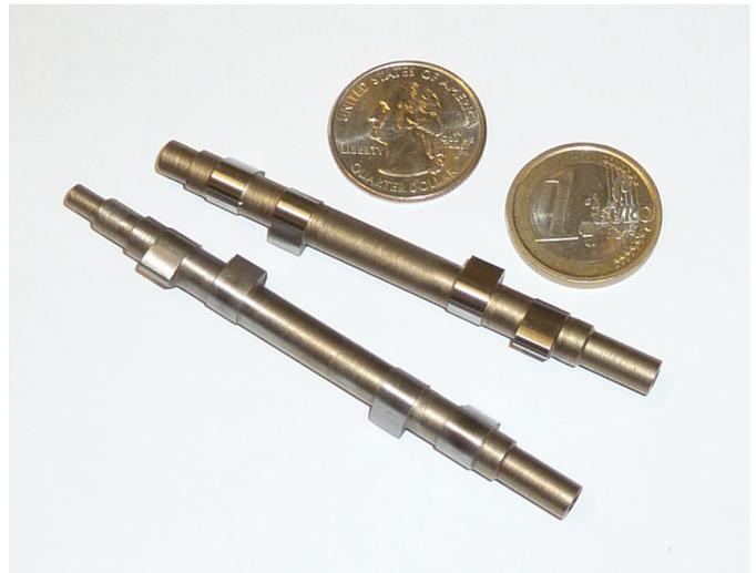
*These are the camshafts that were produced while writing these instructions; however, the shaft ends haven't been ground to size yet.*
